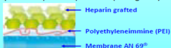
Figure 1 - Structure of oXiris™ membrane.
