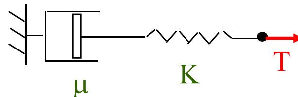
$$\begin{aligned} T &= \mu \dot{d}_1 = K d_2 \\ d &= d_1 + d_2 \end{aligned}$$
