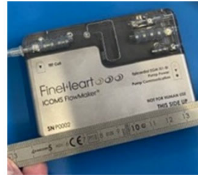
ITC: internal therapy controller 90x65x16mm
