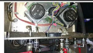
Figure 4. Location of the gaps in the water tank top plates that contributed to the release of aerosols from the heater-cooler unit studied by Public Health England, Porton Down, UK.
